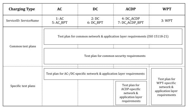
Figure 1 — Overview of relevant conformance test plans for ISO 15118-20 per charging type
